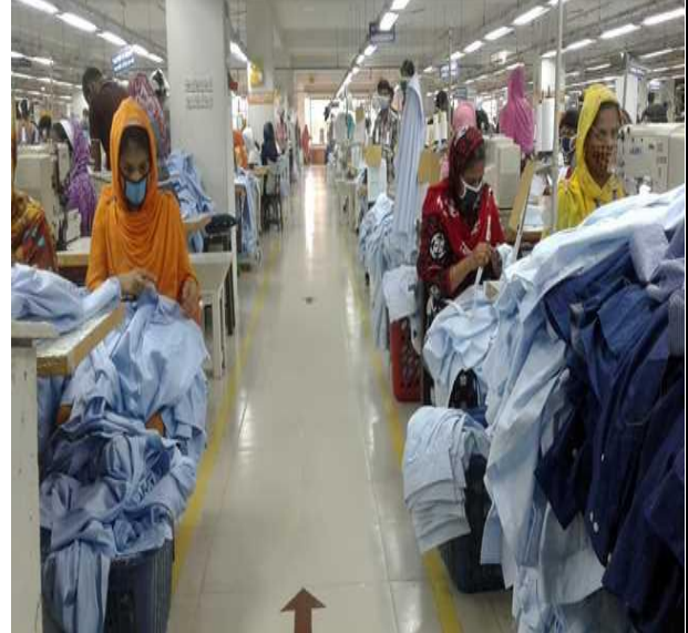
Obstacle/blockage free walkway and no workers are working standing in the walkway.
