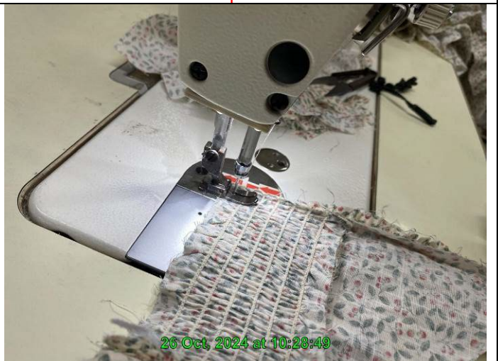
NC# 3.4.9 (b)_ Sewing machine needle guard was missing
