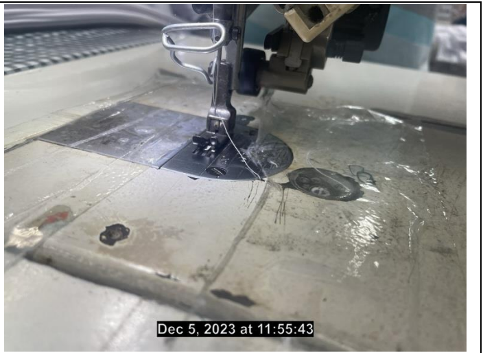
NC# 3.4.9 (b): Needle guard of machine displaced
