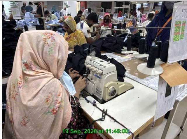
NC_3.4.9 (b): Overlock machine eye guard was displaced
