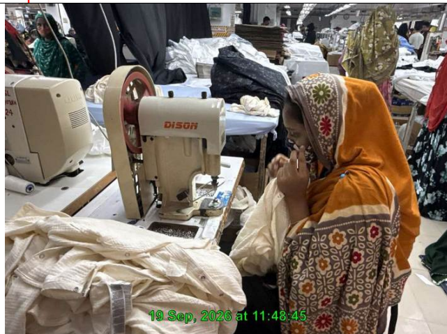
NC_3.4.9 (b): Snap button attach finger guard in active
