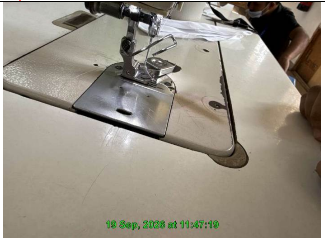
NC_3.4.9 (b): Sewing machine needle guard was displaced
